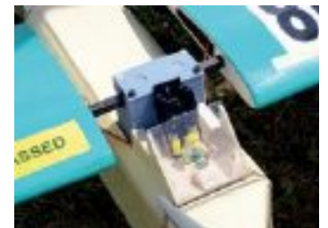
Computer printed folding wing mechanism on City University of London's 'Ball Boys' team Q08 entry. Plus Lego Hans Moleman pilot clutching a void Driving Licence...
