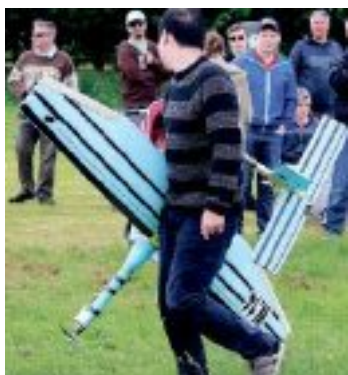
W14 Coventry Uni's Engineering Dept 'Phoenix 1' team's large slender craft was made of blue foam, balsa and black electrician's tape. This was the result of trying to carry 3kg on Sunday.
